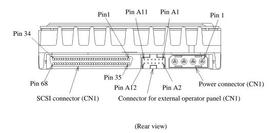
Figure A.2 Locations of connectors and setting terminals (MP model)
